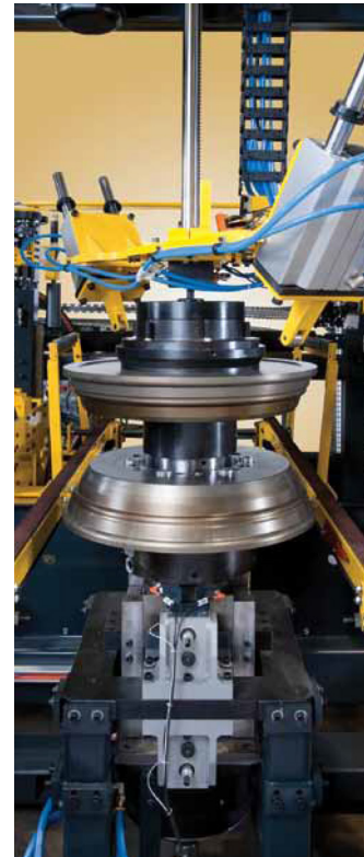
Spindle with measurement devices and transfer conveyor are the heart of the system
